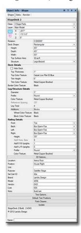
Class, Layer, X, Y, Z, and Rotation: Settings similar to other Vectorworks® symbols and objects. ("Z" is the distance from the drawing's ground plane to the bottom of the StageDeck 2 instance.)
