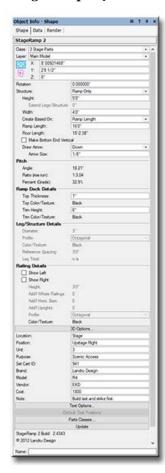
Class, Layer, X, Y, Z, and Rotation: Settings similar to other Vectorworks® symbols and objects. ("Z" is the distance from the drawing's ground plane to the bottom of the *StageRamp 2* instance.)
