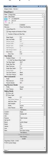
Class, Layer, X, Y, Z, and Rotation: Settings similar to other Vectorworks® symbols and objects. ("Z" is the distance from the drawing's ground plane to the bottom of the StageSteps 2 instance.)
